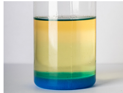
Before. This way water accumulates at the bottom of the tank, causing corrosion.
