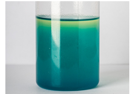
After. The additive combines water and fuel into a microemulsion that burns when the engine runs.
